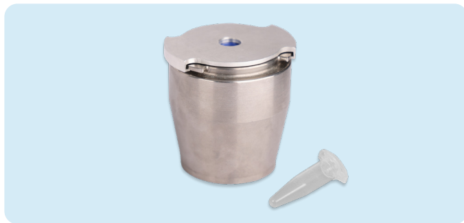
3. Deliver QC sample in a shielded pig
